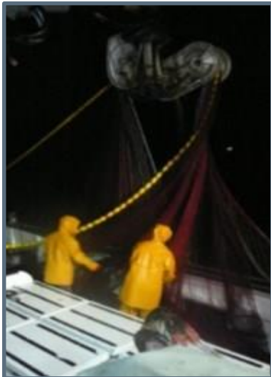
Figure 2.4.3 Purse-seine nets are hauled back on-board with a crane.
