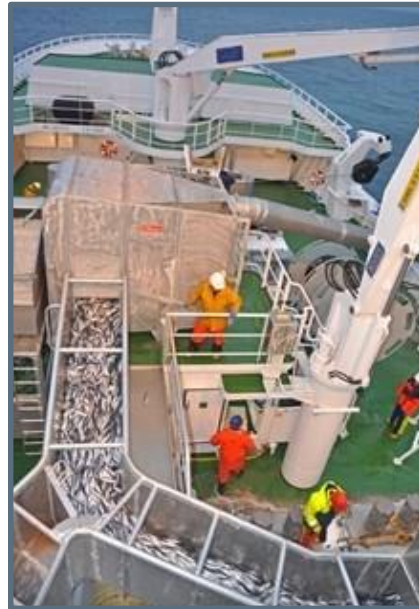
Figure 2.2.4 Catch being pumped through the separator to the RSW tanks.
